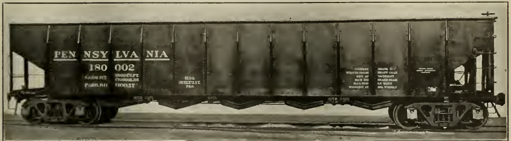
EIGHTY-FIVE-TON, HIGH-SIDE, HOPPER-BOTTOM STEEL GONDOLA BUILT AT ALTOONA, PA., BY THE P. R. R.
